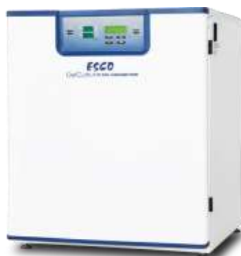
Fig. 1. The CelCulture® CO 2 Incubator with Integrated Cooling System for fish stem cell culture.
